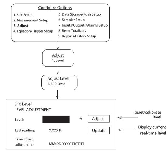
Figure 2-15Ultrasonic level adjustment and calibration
