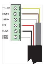
Figure 2-3TIENet Device terminal connections
