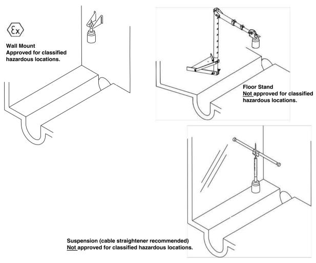
Figure 2-7Sensor mounting options
