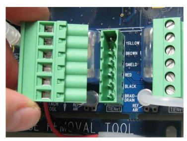
Figure 2-1TIENet Device terminal strips
