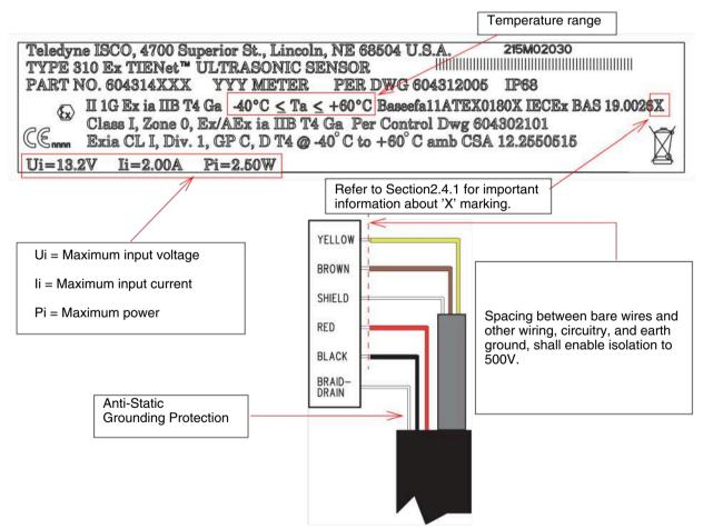
Figure 2-8 Sensor labeling regarding hazloc installations
