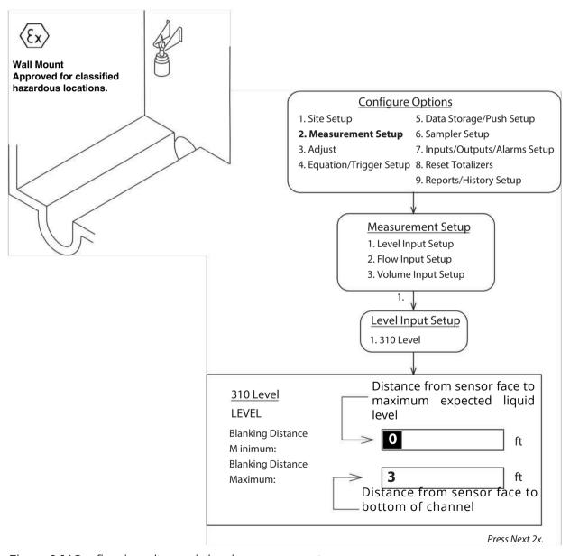
Figure 2-14Configuring ultrasonic level measurement
