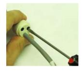
Figure 4-14Removing the plug
