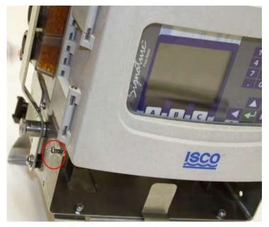
Figure 4-30ne of the eight screws loosened.
