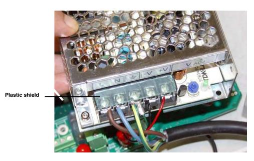
Figure 5-4Power supply terminal strip: AC Input and DC Output
