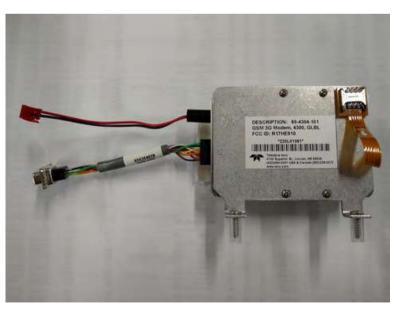
Figure 5-37 GSM Cellular modem-
