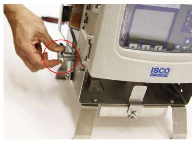
Figure 4-2 Pull out the handle latch pins on each side of the stand
