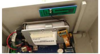
7. Plug the antenna into the antenna plug.
