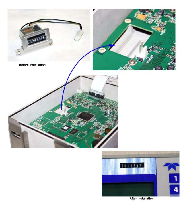
Figure 5-11 Optional non-resettable totalizer installation
