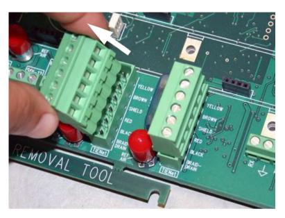
Figure 2-5TIENet Device terminal strips
