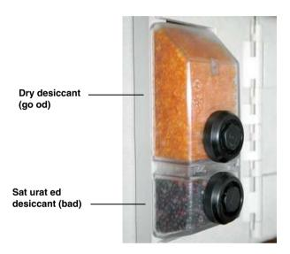
Figure 4-1Desiccant indicating saturation
