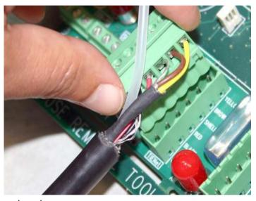
Figure 2-8Attach wired terminal strip to case board socket
