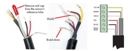
Figure 2-7TIENet Device terminal connections
