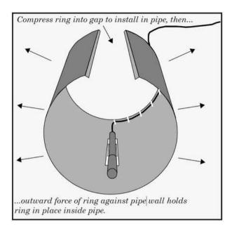
Figure 2-11Sensor Installed on a Spring Ring
