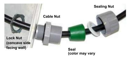
Figure 2-6Installing cable with a cord-grip fitting
