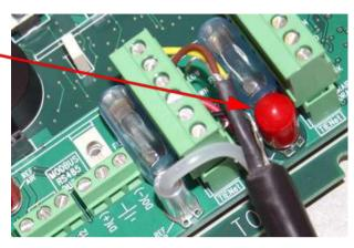
Figure 2-9 Insert the cable reference tubing into the case board reference port
