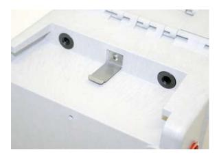
Figure 4-2Removing the external desiccant cartridge
