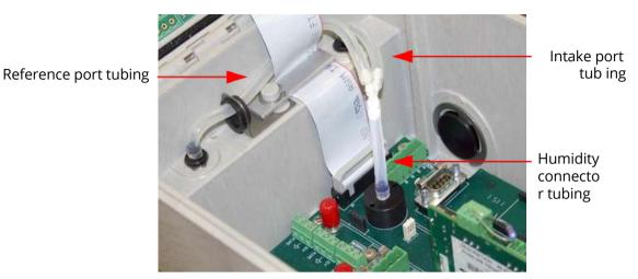
Figure 2-4Tubing configuration for optimal drying power
