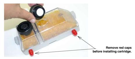
Figure 4-3Opening the desiccant cartridge chambers
