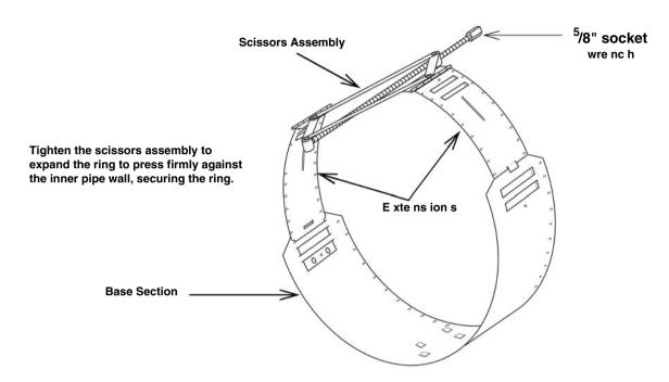
Figure 2-12Scissors Ring adjustment
