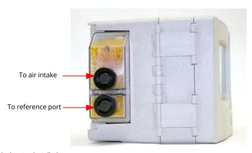
Figure 2-3External desiccator, installed
