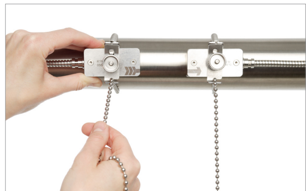
Transducers mounted using chains and clips
