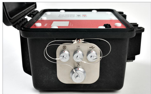
KATflow 210 output connectors
